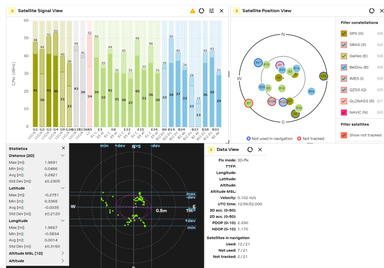
Figure 21. GNSS position analysis using the Taoglas GNSS antenna.
