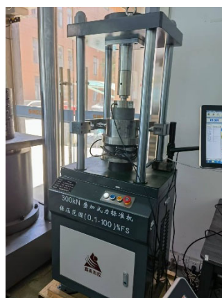
Figure 9. Physical diagram of standard dynamometer and loading verification device.
