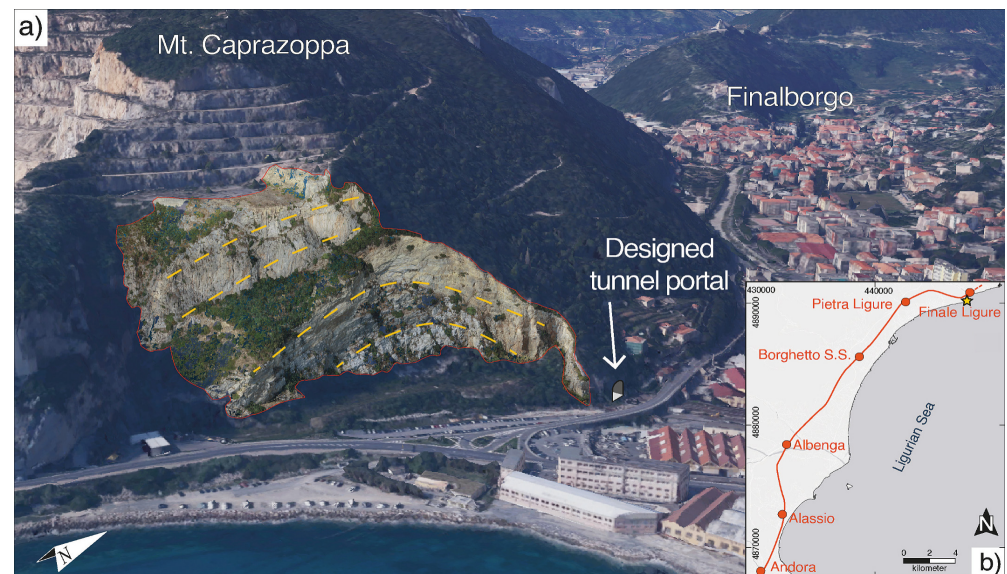
Figure 10. (a) DOM perspective view; red line represents RTK UAV photogrammetric survey area, yellow line represents local fold geometry (b) Path of the new rail line from Finale Ligure Marina to Andora; red circles represent train stops, yellow stars represent DOM locations [66].
