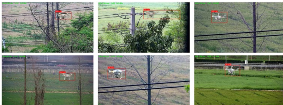
Figure 6. Zero-shot UAV detection results. Example frames illustrating accurate UAV localization (red boxes) across diverse viewpoints and background conditions. The results demonstrate the model’s capability to detect UAVs against complex backgrounds (e.g., trees, fields) without confusion.
