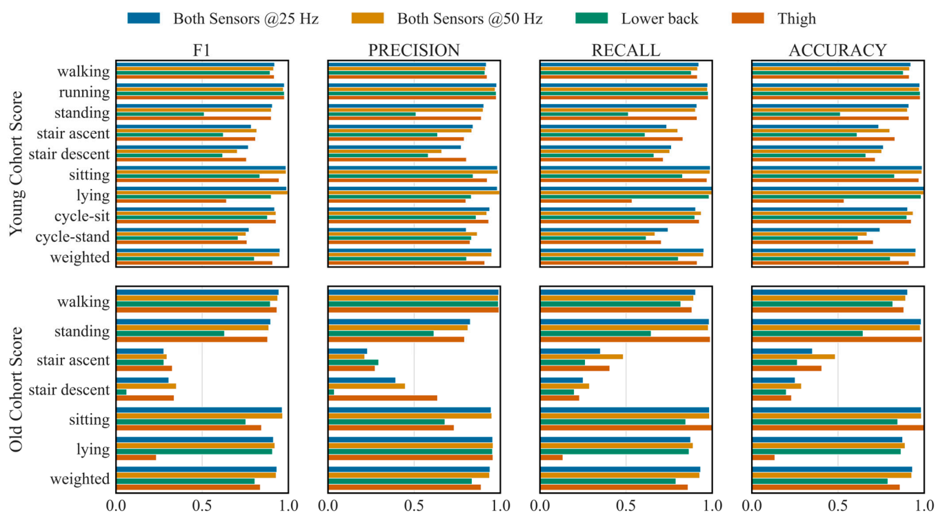
Figure 3. F1-score, precision, recall and accuracy on the Young and Old Cohort Datasets for different experiments (sampling frequency and sensor location). Neural network architecture and hyperparameters were optimised for each experiment. The metrics per activity and their average weighted by their frequency (“weighted”) are presented.
