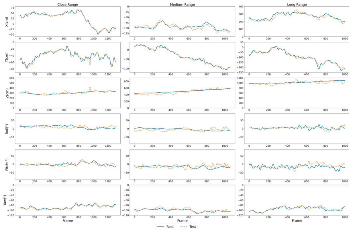
Figure 9. Comparison curves between the estimated and ground-truth 6-DoF position and orientation in three scenarios. The blue curves indicate the ground truth, and the orange curves indicate the estimated results. The X, Y, Z, and yaw components exhibit close tracking between estimation and ground truth across all scenarios, while relatively larger deviations are observed in the roll and pitch components.
