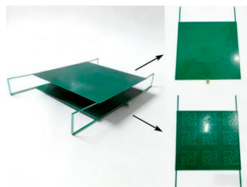
Figure 13. Physical diagram of the Koch fractal antenna.
