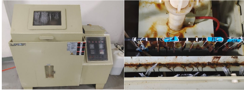
Figure 2. Salt spray test chamber and specimen placement.
