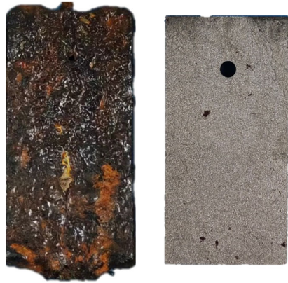
Figure 3. Before (left) and after (right) removal of corrosion products.
