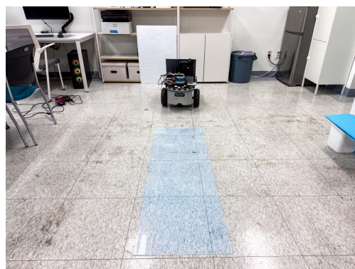
Figure 7. Narrow indoor experimental environment incorporating an extremely low-friction surface.
