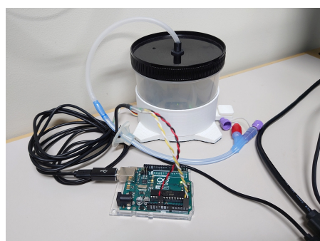
Figure 3. A sensing device used to measure the dosing rate in ESTE-TF.
