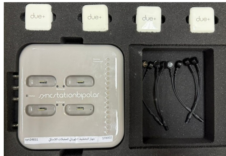
Figure 1. OT Bioelettronica DUE+ wireless sEMG acquisition system (OT Bioelettronica, Italy). The sync station/charger is shown on the left, and the wireless bipolar probes with electrode leads are shown on the right. The non-English label on the device identifies the wireless EMG acquisition system.
