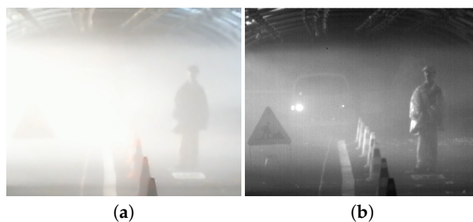
Figure 1. Artificial fog conditions during daylight at the Cerema’s PAVIN platform [8]. The same scene is captured (a) in the visible spectrum (0.38–0.75 \mu\text{m} ), and (b) in the Short-Wave Infrared (SWIR) spectrum (0.9–1.7 \mu\text{m} ). Reproduced from [9].
