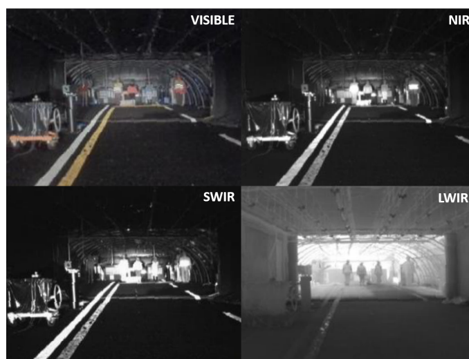
Figure 2. Visual comparison of the same scene captured in four spectral bands: Visible (VIS), Near-Infrared (NIR), Short-Wave Infrared (SWIR), and Long-Wave Infrared (LWIR). The figure illustrates the differences in appearance, contrast, and detail visibility across these modalities. Images acquired by Cerema as part of the FUI AWARE project. Adapted from [11].
