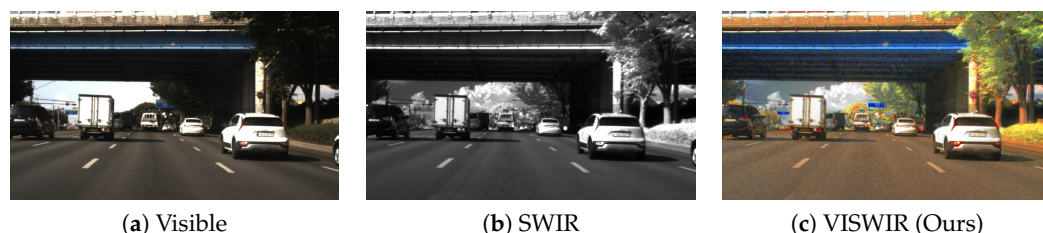
Figure 8. Qualitative evaluation on the RASMD dataset in a high-dynamic-range scenario. The visible image (a) suffers from underexposure under the bridge, while the SWIR image (b) highlights the high reflectance of the vegetation. The IQA-optimised VISWIR fusion (c) integrates both, recovering details in deep shadows without saturating the bright areas.
