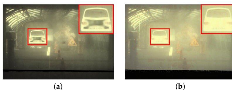
Figure 4. Visual comparison of pseudo-RGB images from our VISWIR method before (a) and after (b) post-processing. The latter shows enhanced visual quality, with improved local contrast, sharper details and reduced artefacts, while preserving the natural colour rendering of the fused image. The red boxes highlight specific regions where these structural and contrast enhancements are most prominent.
