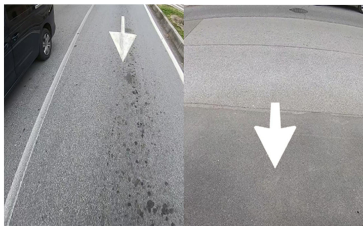
Figure 8. Comparison between real (left) and synthetic (right) horizontal road marking samples. The synthetic sample was generated by superimposing a digital marking template onto a real pavement background while varying scale, orientation, and perspective.
