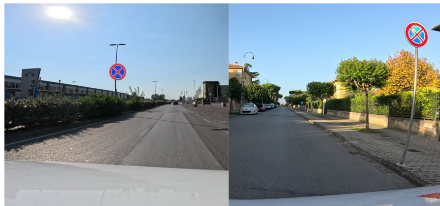
Figure 6. Comparison between synthetic (left) and real vertical traffic sign (right) samples. The synthetic example was generated by superimposing a digital sign template onto a real road background, while the real example was extracted from the acquired survey footage.
