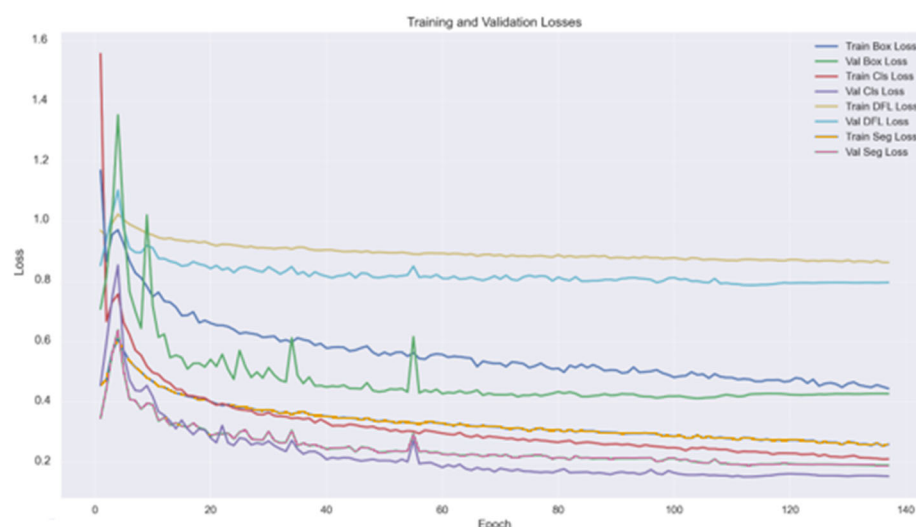
Figure 10. Training and validation loss curves of the YOLO11m-seg model selected for horizontal road marking segmentation. The plot reports box loss, classification loss, distribution focal loss (DFL), and segmentation loss for both training and validation over the training epochs.
