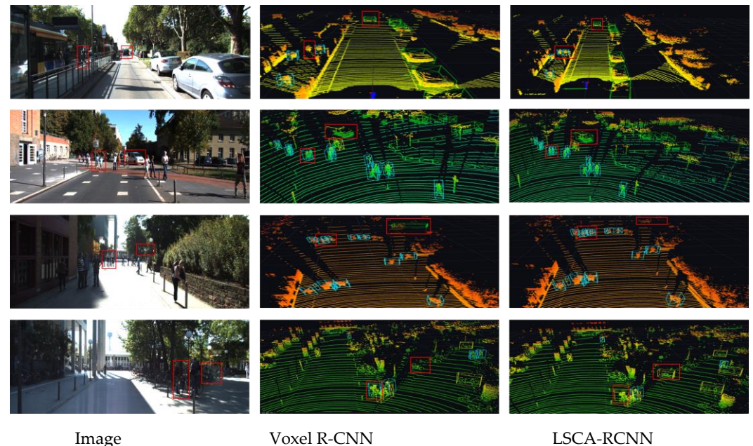
Figure 5. Visualization of detection results on the KITTI dataset. Blue boxes represent pedestrians, yellow boxes represent cyclists, and green boxes represent vehicles. The red box denotes the comparison region.
