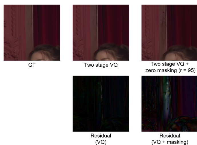
Figure 10. Visual comparison of the proposed two-stage VQ method without and with zero-masking on the Bartender dataset for View 6. The comparison is performed before HEVC video coding and shows only the VQ-based reconstruction results. The second stage uses nine residual sub-vector groups, and the zero-masking ratio is set to 0.95. The top row shows the rendered images, while the bottom row presents the corresponding residual maps with respect to the reference rendering.
