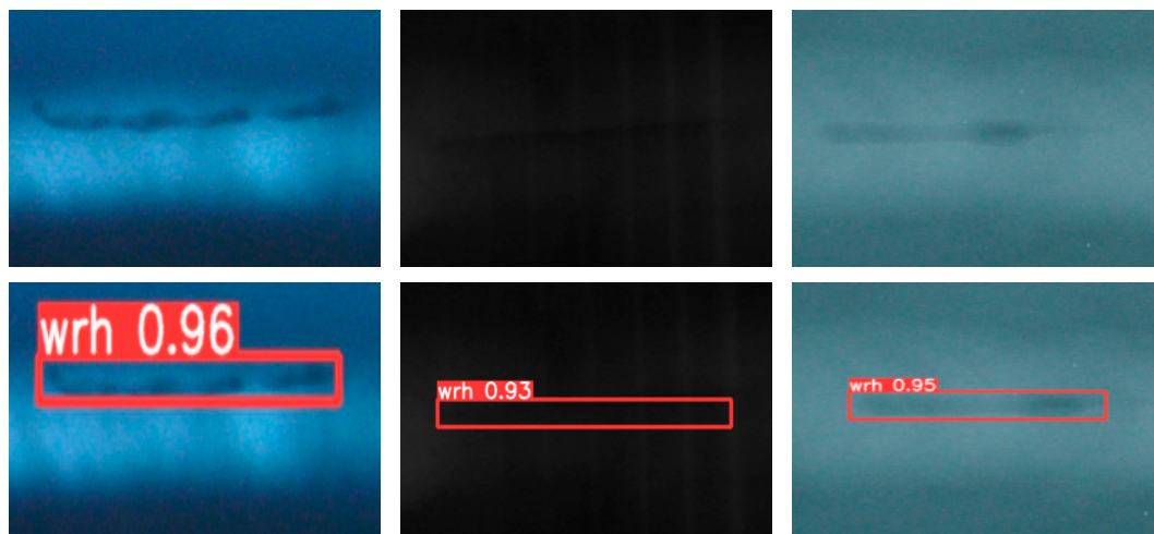
Figure 18. Example of lack of fusion recognition.
