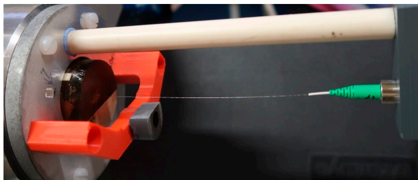
Figure 12. Photograph of the sapphire fiber exiting the epoxy target at the end of the gas launcher.
