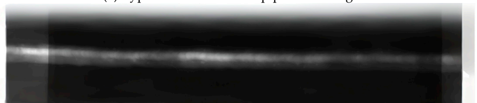
(b) Typical image of a long-distance pipeline weld.
