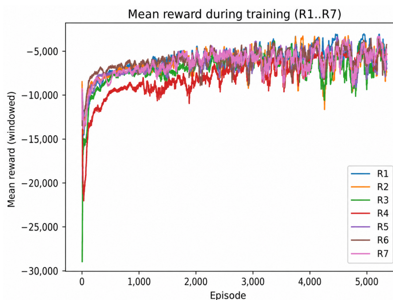
Figure 2. Mean episode reward during PPO training for reward variants R1–R7. Higher values, i.e., values closer to zero, indicate better policy performance because the reward function is composed primarily of penalty terms.
