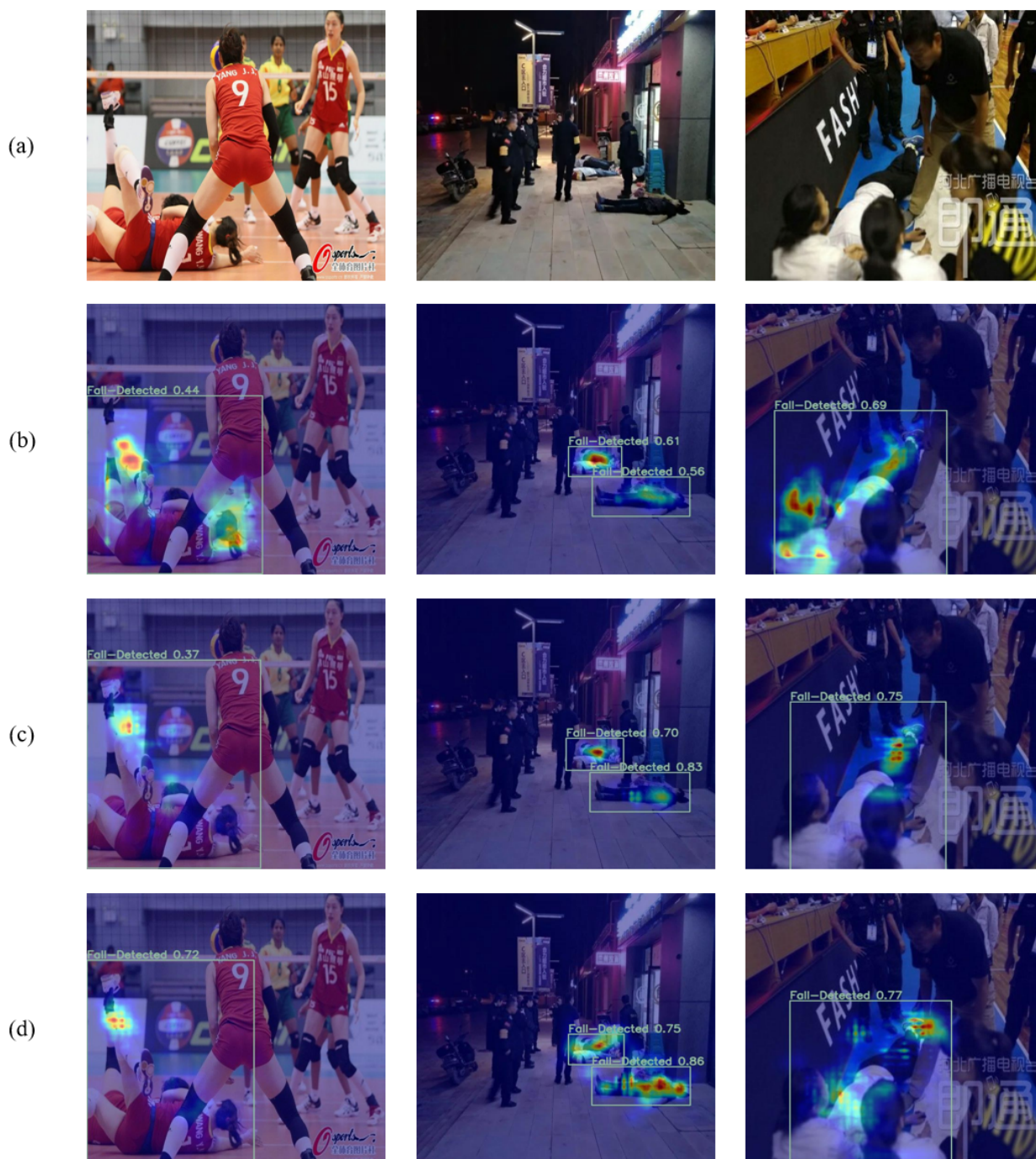
Figure 6. Comparison of model inference heatmap. (a) Ordinary images, (b) YOLOv11n heatmaps, (c) YOLOv8n heatmaps, (d) WAD-YOLO heatmaps. From left to right are ordinary scene, multi-objective scene and the scene where the target is blocked. In the heatmaps, red regions indicate high activation areas where the model focuses its attention, while blue regions indicate low activation areas with minimal model response.
