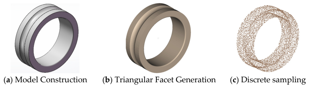
Figure 8. Construction Process of the Bearing Ring Dataset.
