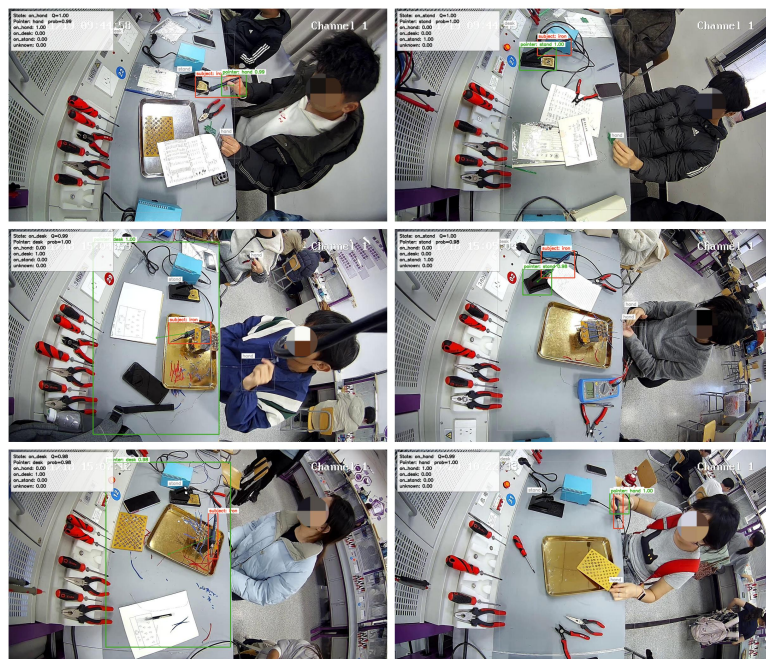
Figure 9. Visualization of RISNet intermediate outputs. Each example shows the soldering iron subject, candidate environmental objects, the object selected by Pointer-Head, state probabilities from State-Head, and the reliability score from Quality-Head.
