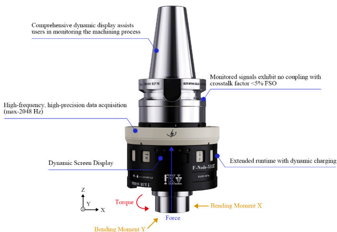
Figure 1. Advantages of the wireless smart toolholder.
