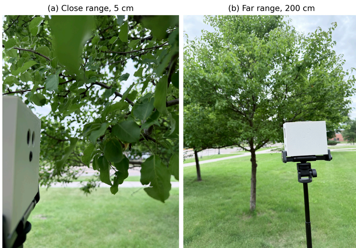
Figure 8. Field measurement setup on a live tree canopy in Brookings, SD: (a) close range, 5 cm, with foliage filling the sensor field of view; (b) far range, 200 cm.
