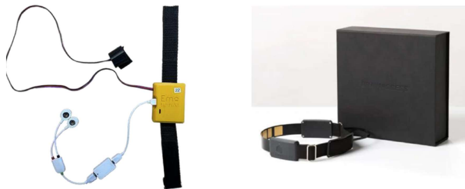
Figure 4. Physiological signal collection devices used in the SonikB3D project, ( left ) ScientisSt-EMOTIPHA sensor; ( right ) BrainAccess HALO.
