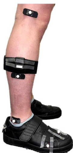
Figure 1. Placement and fixation of the wearable posture sensor on the shank segment. The sensor was attached to the lateral aspect of the shank and secured using an elastic Velcro strap, double-sided adhesive tape, and additional surgical tape to minimize relative motion between the sensor and skin during walking.
