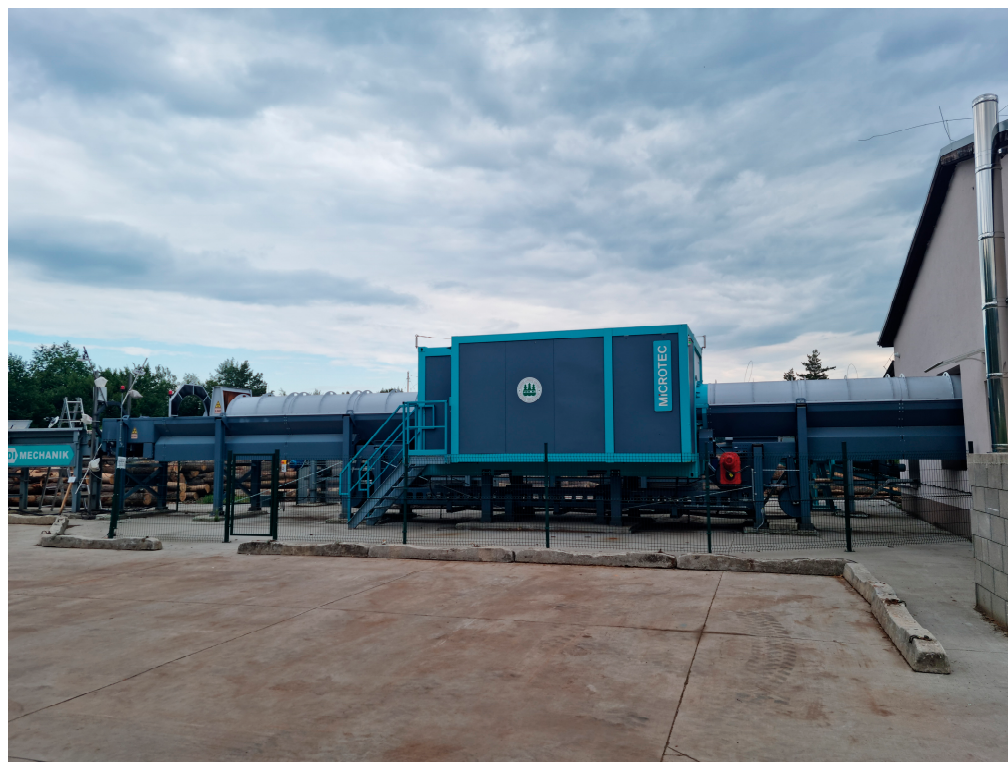
Figure 2. Three-dimensional CT scanner manufactured by Microtec based in Italy.
