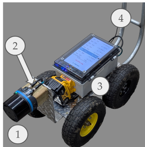
Figure 1. Single-operator push-cart platform for plot-scale LiDAR phenotyping. The cart carried a (1) SICK multiScan136 multi-beam time-of-flight LiDAR mounted horizontally 0.39 m above the ground, (2) an inertial measurement unit for roll and pitch correction, and a wheel encoder for distance tracking. A Raspberry Pi 5 (3) recorded the LiDAR data stream, while a Raspberry Pi Pico 2 recorded encoder counts and IMU orientation. Both data streams were synchronized using a shared pulse-per-second signal from a DS3231 real-time clock. Data collection was controlled with a handle-mounted (4) logging button and a custom Python v3.11 interface that selected the experiment, started and stopped scans, and saved paired LiDAR and microcontroller files for each plot.
