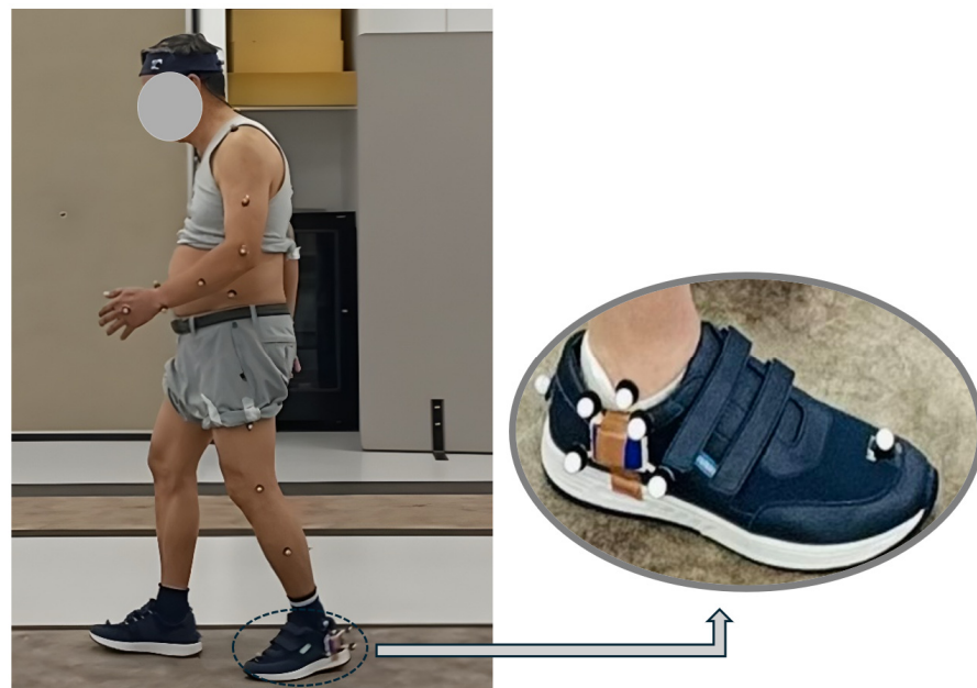
Figure 1. Participant performing a walking trial with reflective markers and IMUs attached. The inset depicts the placement of the Vicon IMU and the attached marker cluster.
