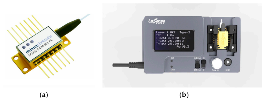
Figure 3. Laser source: (a) EP1392-DM-B semiconductor laser; (b) M01 laser driver.
