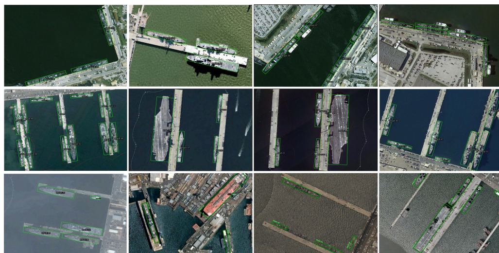
Figure 4. Qualitative detection results of SPFDet on the HRSC2016 dataset. The green bounding boxes indicate detected ships. Our method successfully handles challenging scenarios including dense ship clusters, varying scales, and complex harbor backgrounds.
