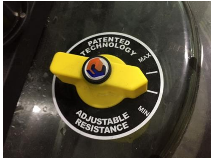
Figure 2. Apollo AR water-resistance rowing machine and resistance-level controller. The four manufacturer-defined resistance settings were MIN, Level 2, Level 3, and MAX.
