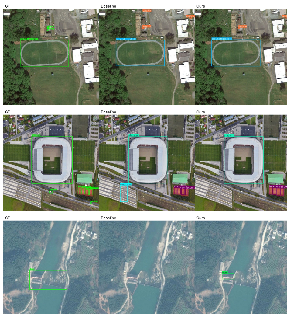
Figure 10. Typical failure cases of the proposed method in complex optical remote sensing scenes. The frame colors are automatically assigned according to object categories by the visualization tool, and the category names are shown next to the corresponding boxes.
