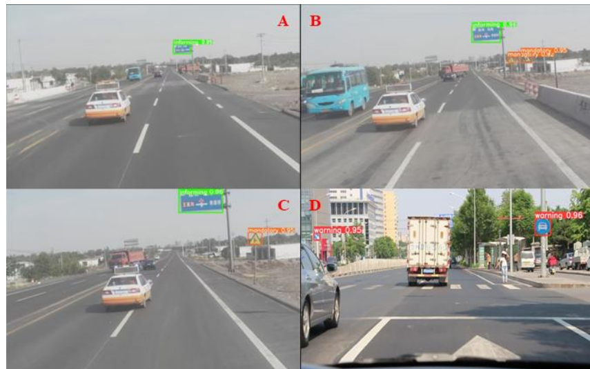
Figure 8. Multi-frame road sign detection performance at varying observation distances. Panels (A–C) demonstrate consistent bounding box alignment as the inspection vehicle approaches an informative sign, while Panel (D) captures a warning sign in a complex urban background (Note: Chinese characters appearing on the road signs in the background are original real-world environment elements, and different bounding box colors are used for visual distinction of target tracking.).
