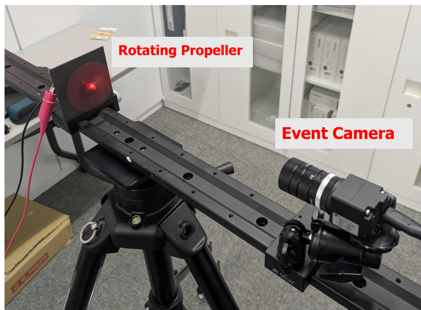
Figure 1. Experimental setup for event-camera-based observation of a high-speed rotating propeller. The main components are labeled in the figure: the rotating propeller, which served as the inspection target, and the event camera. The event camera and the propeller were fixed on the same rail so that the camera faced the propeller from the front and the rotating propeller remained within the field of view throughout the experiment.
