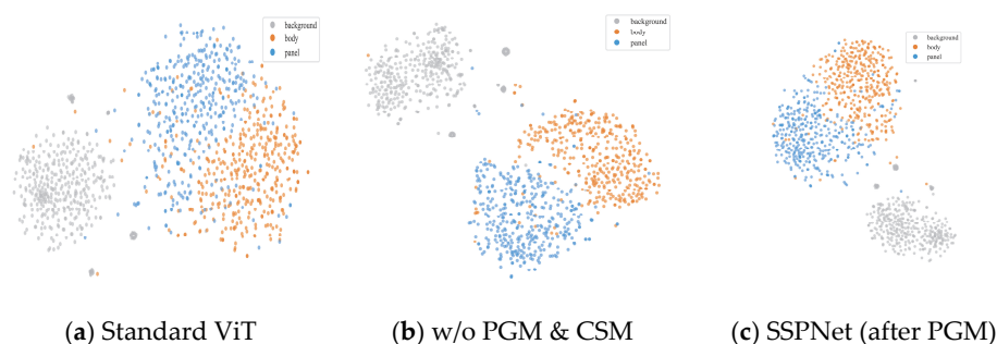
Figure 16. t-SNE dimensionality reduction results. (a) shows the dimensionality reduction result of the standard ViT encoder features; (b) shows the dimensionality reduction result of the GMHC-ViT encoder features; (c) shows the dimensionality reduction result after prior information injection into the GMHC-ViT encoder features.
