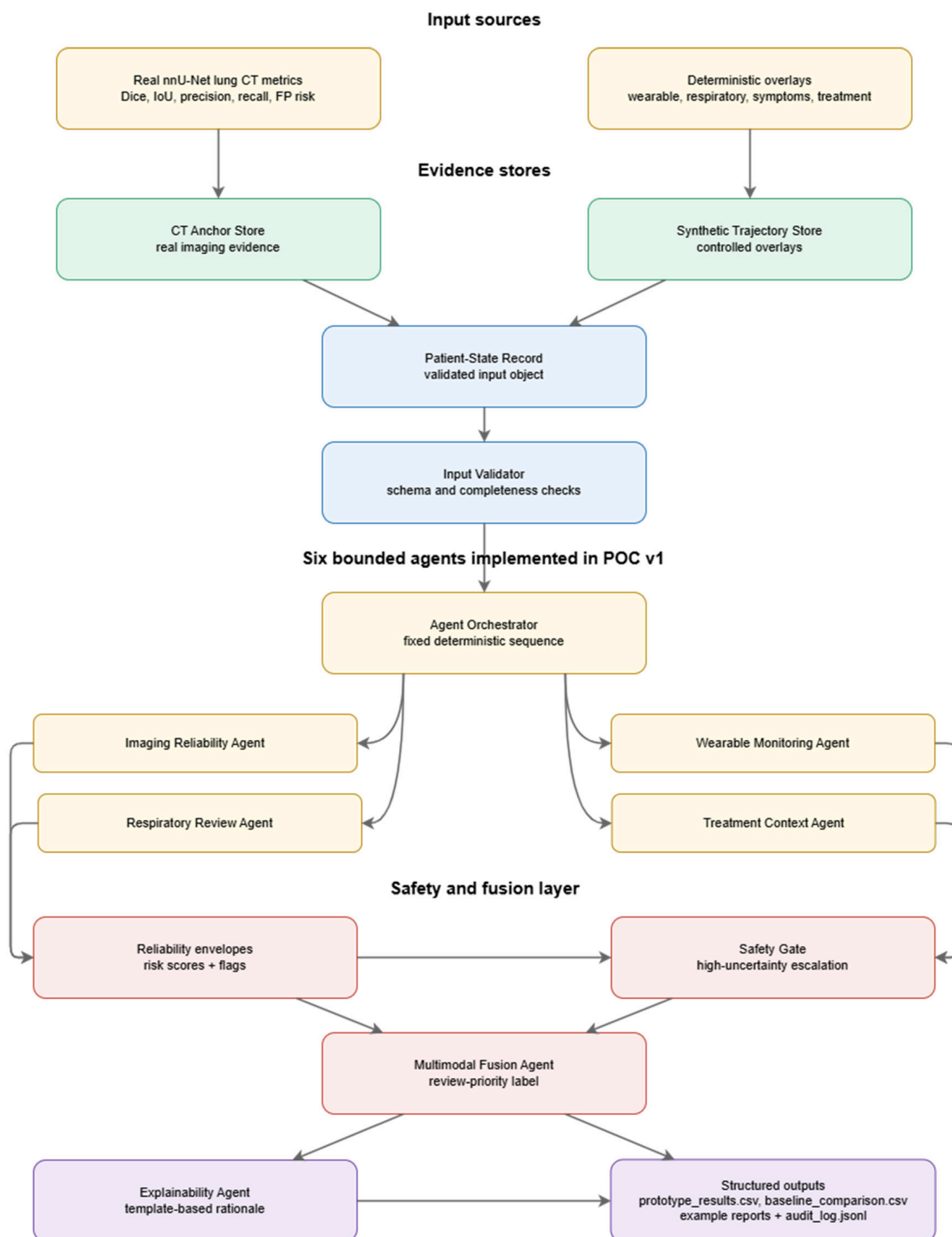
Figure 3. Technical architecture of the OncoSense-Agent POC implementation. Real lung CT segmentation metrics are loaded into the CT Anchor Store, while deterministic wearable, respiratory, symptom, and treatment-context overlays are loaded into the Synthetic Trajectory Store. Validated patient-state records are processed by six implemented bounded agents: Imaging Reliability, Wearable Monitoring, Respiratory Review, Treatment Context, Multimodal Fusion, and Explainability. The Safety Gate converts low reliability or conflicting high-risk evidence into auditable high-uncertainty review states. The pipeline produces structured outputs, including per-patient prototype results, baseline-comparison results, example clinician-facing reports, and an audit log. The remaining five agents from the full eleven-agent architecture are specified for future integration and were not implemented in POC v1.
