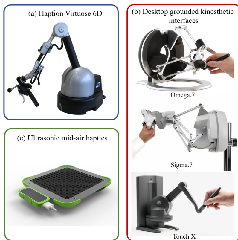
Figure 4. Representative haptic systems used in medical robotics and surgical simulation. (a) Haption Virtuose 6D, a grounded 6-DOF kinesthetic interface capable of rendering forces and torques for teleoperation and simulation; (b) representative desktop kinesthetic interfaces including Omega.7, Sigma.7, and Touch X, commonly used as master devices in surgical simulation and robotic teleoperation; (c) ultrasonic mid-air haptic technology for contactless tactile feedback. These examples illustrate the diversity of current haptic platforms, ranging from high-force kinesthetic systems to lightweight tactile displays [4,15,20].
