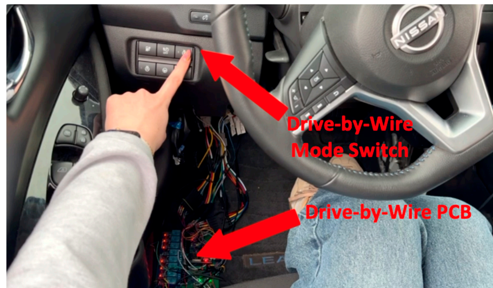
Figure 2. Drive-by-wire retrofit interface steering hardware solution implemented on the 2025 Nissan Leaf test vehicle.
