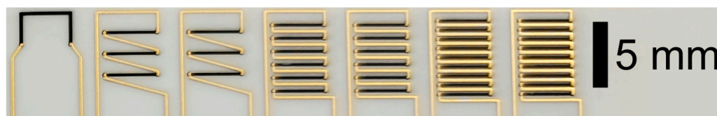
Figure 4. Top part of one sensor substrate with CCO and gold lines already on the substrate. One substrate consists of one sensor with one thermocouple, and two sensors with thermopiles with three, six, and nine thermocouples, respectively.
