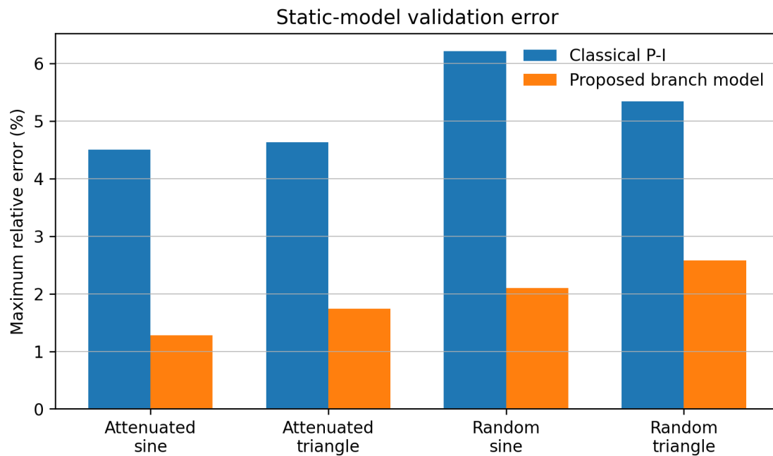
Figure 11. Maximum relative error comparison between the classical P-I model and the proposed branch polynomial model.
