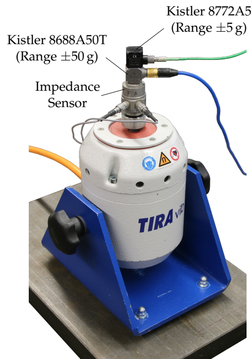
Figure 7. Shaker test setup with two different accelerometers with \pm 5 g and \pm 50 g range.
