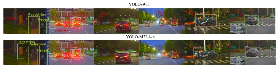
Figure 8. Detection differences between YOLOv9-n and YOLO-M2LA-n.
