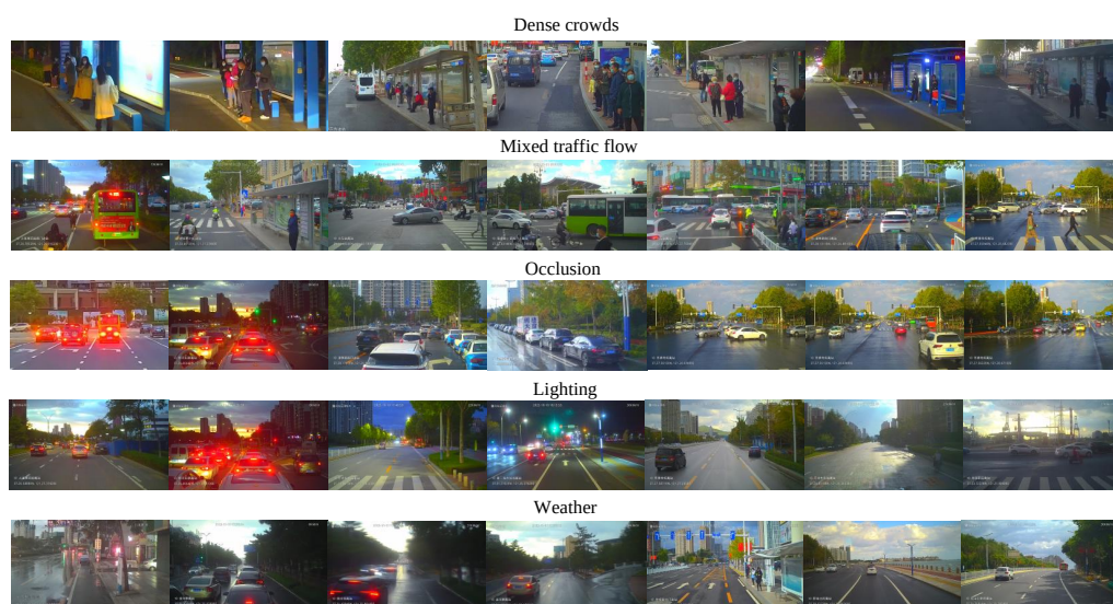
Figure 4. Representative examples from the BFTD under diverse scenarios. The dataset covers visually challenging traffic scenes including dense crowds, mixed-traffic flow, occlusion, illumination variation, and different weather conditions.
