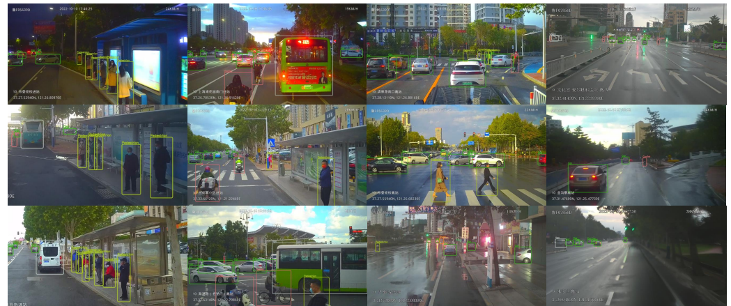
Figure 9. Representative detection results of YOLO-M2LA-x on the BFTD dataset. The model achieves accurate recognition of small pedestrians, riders, and vehicles under dense traffic, frequent occlusion, and varying illumination conditions.
