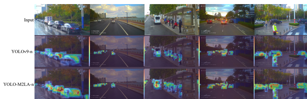
Figure 7. Visualization of Class Activation Maps (Grad-CAM++) comparing YOLOv9-n and the proposed YOLO-M2LA-n on vehicle detection.
