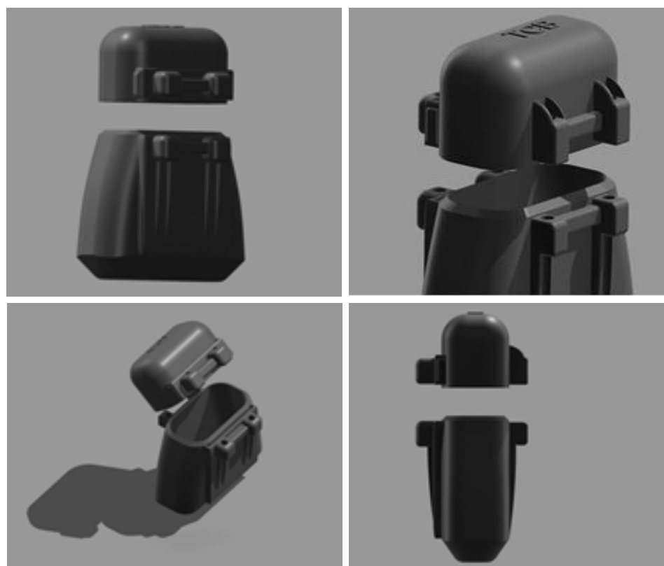
Figure 3. Custom-designed enclosure for the wearable collar, optimized for durability and animal comfort.
