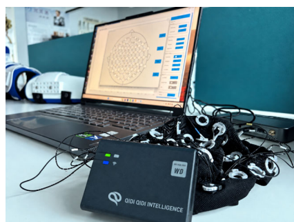
Figure 1. EEG acquisition system and recording interface used for 32-channel recording.
