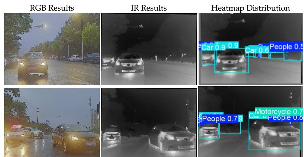
Figure 9. Each row represents a set of RGB, IR, and detection images. The (left) column shows the ground truth RGB image. The (middle) column shows the ground truth IR image. The (right) column shows the detection result of MHF-Net.
