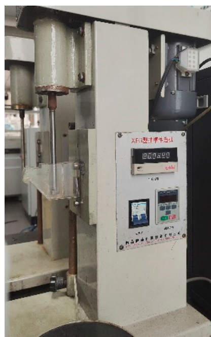
Figure 2. The XFG flotation machine used in the study.
