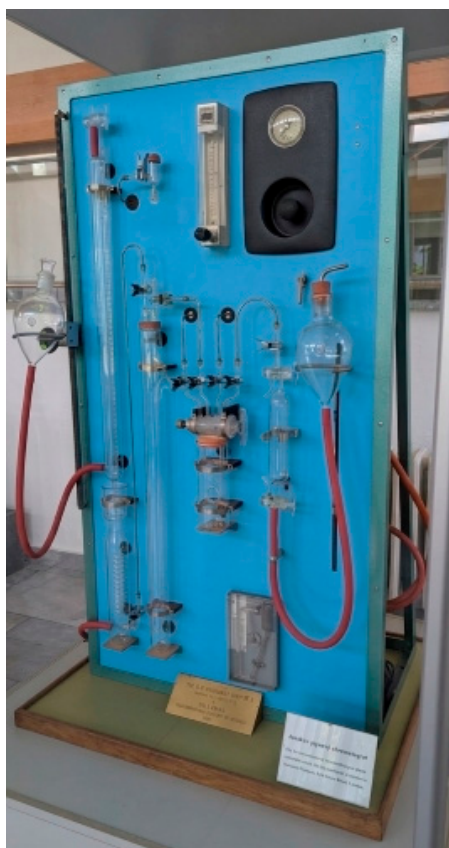
Figure 1. Janak's volumetric gas chromatograph—the instrument is displayed in the vestibule of the building of the Institute of Analytical Chemistry, Czech Academy of Sciences, in Brno.
