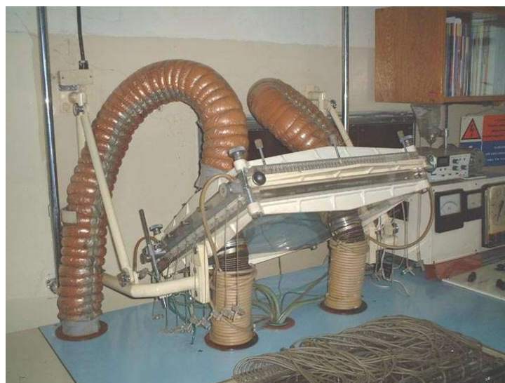
Figure 3. Apparatus for continuous free-flow electrophoresis.
