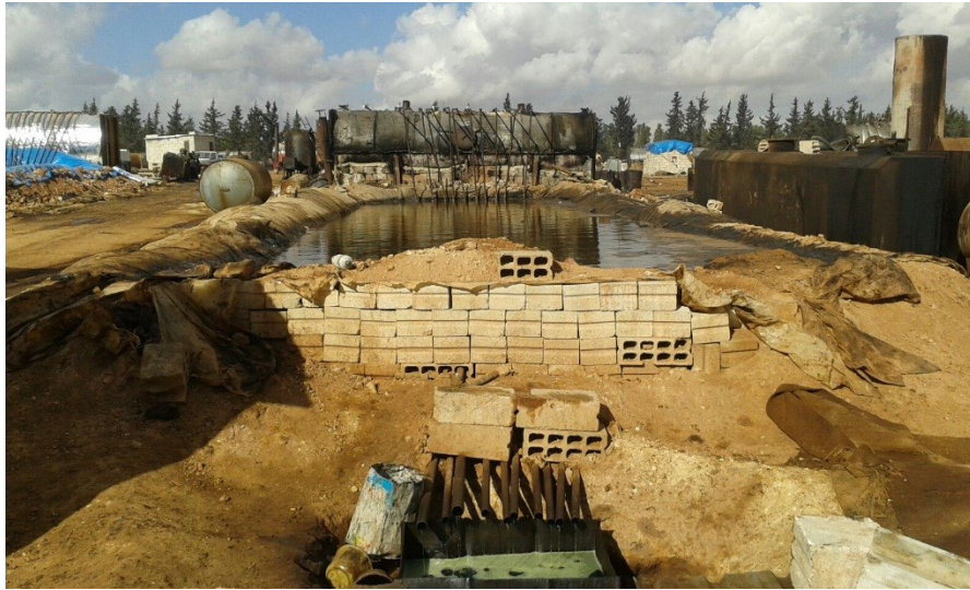
Figure 7. The primitive metal kilns to refine crude oil from Manbij (province Aleppo) into a pit where it will be distilled.
