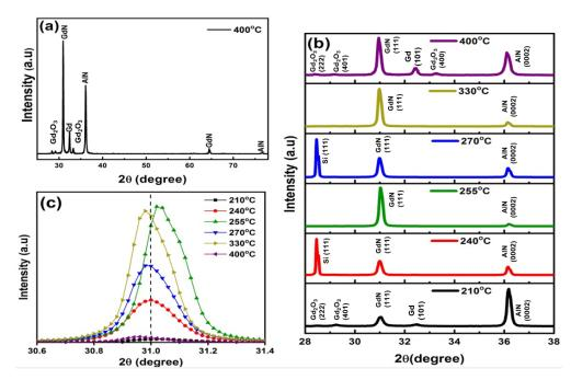
**Figure 4.** XRD pattern of (**a**) 400 °C annealed Gd film grown on AlN (0001) sample, (**b**) comparison of Gd films grown on AlN (0001) samples annealed in different temperature 210 °C, 240 °C, 255 °C, 270 °C, 330 °C and 400 °C, (**c**) showing the shift in the samples at  $2\theta = 31^{\circ}$ .
