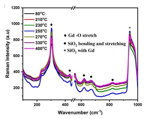
**Figure 5.** Room temperature Raman spectra of samples grown at 80 °C, 210 °C, 240 °C, 255 °C, 270 °C, 330 °C and 400 °C. A break is done from 450 cm $^{-1}$  to 550 cm $^{-1}$  to avoid the Si strong peak.
