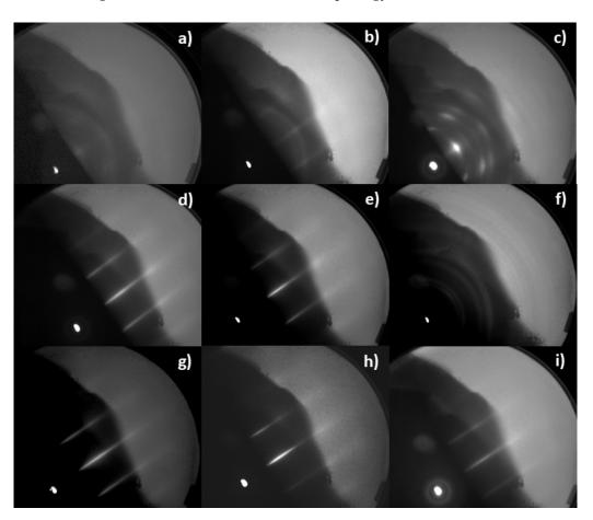
**Figure 3.** RHEED images of (a) 80 °C, (b) 210 °C, (c) 210 °C rotated 90°, (d) 240 °C, (e) 255 °C, (f) samples after 30 min annealing at 255 °C, (g) 270 °C, (h) 330 °C and (i) 400 °C films grown on AlN (0001) samples.
