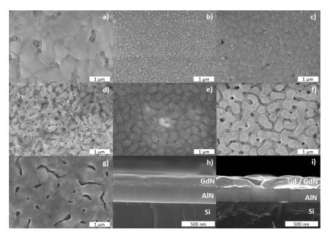
**Figure 1.** Secondary electron SEM mages of (a) 80 °C, (b) 210 °C, (c) 240 °C, (d) 255 °C, (e) 270 °C, (f) 330 °C and (g) 400 °C Gd films grown on AlN (0001) samples and cross sections of the (h) 330 °C and (i) 400 °C films. Cross sections were prepared by inducing a clean fracture in the underlying Si wafer.
